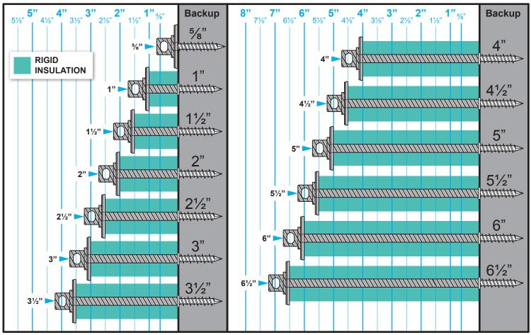
**THERMAL Concrete Seal Tie™** is an innovative single screw veneer tie suitable for use with concrete, CMU, wood stud, or brick backup. (for wood stud refer to wood stud size and selection chart)
