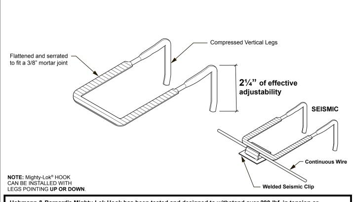
Hohmann & Barnard's Mighty-Lok Hook has been tested and designed to withstand over 290-lbf, in tension or compression, at maximum allowed offset (TMS 402/602-16 12.2.2.5.5.4) of 11/4" (disengagement of the pintle from the veneer anchor). These results exceed BIA recommendations and the capabilities of standard "round wire" hooks/pintles by over 100%, while maintaining the ASTM A1064/1064M wire specification.
