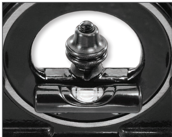
Close-up of spirit level on back side of protractor
