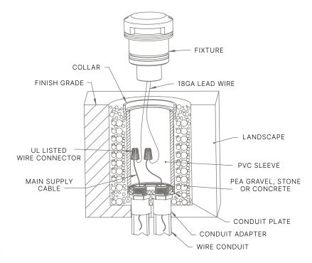
TIP: Small gauge cable is vulnerable to damage in the landscape; Protect by routing in close proximity to the luminaire or adjacent to concrete slab or similar structure. Do not over tighten.
