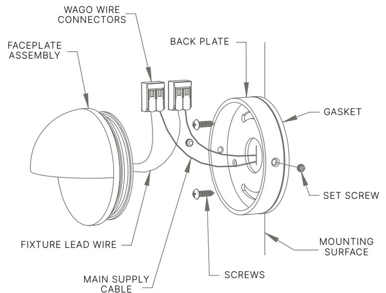
**TIP:** Small gauge cable is vulnerable to damage in the landscape; Protect by routing in close proximity to the luminaire or adjacent to concrete slab or similar structure. Do not over tighten.
