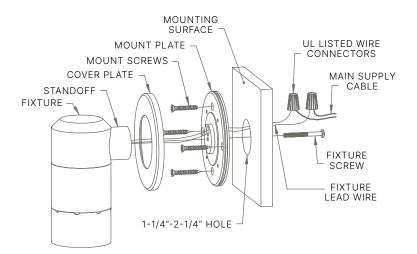
**TIP:** Small gauge cable is vulnerable to damage in the landscape; Protect by routing in close proximity to the luminaire or adjacent to concrete slab or similar structure. Do not over tighten.
