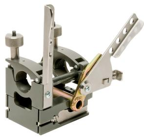
An alternative to the Mini-Mc®, the 1LC offers a more conventional style of operation while maintaining the great features of the 2LC. The heater is designed to locate on the guide rods of the unit, similar to most other McElroy fusion machines. The 1LC's compact design also allows for fusing in tight quarters.
