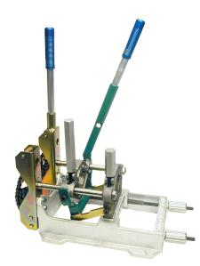
The 2CU will butt fuse ½" CTS to 2" IPS (16mm to 60mm) pipe, tees, ells and other fittings. This combination unit (CU) incorporates McElroy's patented sidewall feature. Sidewall clamps with chain vise allow the unit to be attached on the centerline of a pipe main for sidewall fusion of ½" to 2" service saddles, round base branch saddles and small tapping tees. The 2CU is equipped with chain lengths that will clamp up to 8" IPS pipe. Additional chain lengths are available for larger main sizes.
