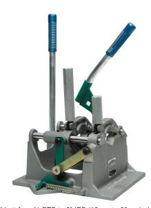
The 2LC will butt fuse ½ CTS to 2" IPS (16mm to 60mm) pipe. By employing a semi-automatic locking cam (LC) system, the 2LC expertly maintains force during the cooling cycle.
