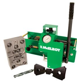
The In Field \* Tensile Tester provides a quick and easy way to qualitatively test fusion joints in the field. Dual reduced section coupons allow for quick comparisons between integrity of the joint and the parent pipe. A hand-pump system tests coupons from 2" IPS and larger pipes (up to 5" thick wall).
