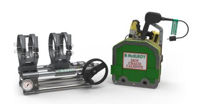
The Polygon allows installers the flexibility to complete butt and miter fusions from zero- to 45-degree angles for 2" to 6" (63mm to 180mm) polyethylene pipe. It has the additional capability to perform socket fusions for 2" to 4" (63mm to 125mm) polyethylene pipe and fittings.
