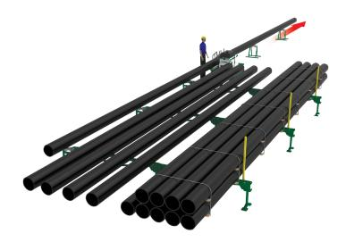
The McElroy PolyHorse <sup>®</sup> is a pipe-handling system that consists of a series of adjustable racks to store and help install pipe on the jobsite. For use with polyethylene pipe sizes from 3" to 20", the PolyHorse can reduce labor expenses by providing an efficient, less hazardous work environment for handling pipe bundles and enhance jobsite productivity.
