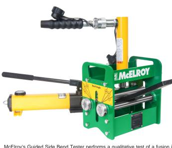
McElroy's Guided Side Bend Tester performs a qualitative test of a fusion joint by destructively testing a coupon. The quality assurance device tests the ductility of polyethylene pipe fusion joints in a safe, quick manner. This testing method places the entire wall thickness into tension and gives assurance of the ductility of joints.
