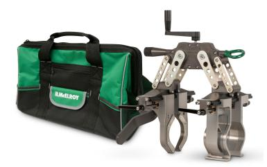
The Spider <sup>™</sup> 125 Series 2 is the preferred equipment for quick and accurate socket fusion of polypropylene pipe and fittings from 63mm to 125mm. Only one operator is required to efficiently align, heat, fuse and cool the pipe. With a lightweight and compact design, the Spider is ideal for performing socket fusions overhead, vertically and other tight indoor spaces from the attic to the floor.
