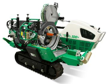
McElroy's TracStar  $^{\circ}$  500 Series 3 will butt fuse pipe sizes from 6" IPS to 20" OD (160mm – 500mm). In 1997, the TracStar 500 debuted as the world's first self-contained, self-propelled, all-terrain fusion machine. Considered the flagship McElroy fusion machine, the success of the TracStar 500 spawned the entire TracStar line of fusion equipment.
