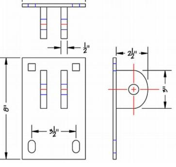
The female has two  $\frac{1}{2}$ " tabs with holes that will fit a  $\frac{3}{4}$ " bolt or pin, and would be used on an 8" Truss Frame.
