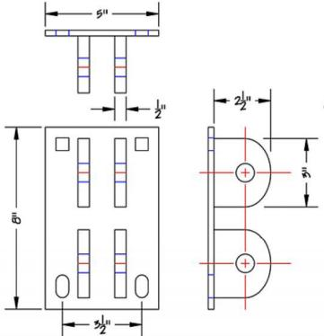
The female has four  $\frac{1}{2}$ " tabs with holes that will fit a  $\frac{3}{4}$ " bolt or pin, and would be used on an 8" Truss Frame.
