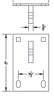
The male has one  $\frac{5}{8}$  tab with a hole that will fit a  $\frac{3}{4}$  bolt or pin, and would be used on an 8 Truss Frame.
