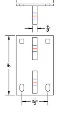
The male has two  $\frac{5}{8}$ " tabs with holes that will fit a  $\frac{3}{4}$ " bolt or pin, and would be used on an 8" Truss Frame.
