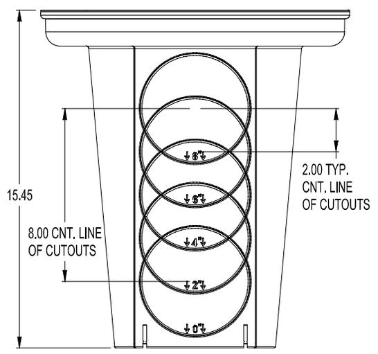
HOLES TO BE CUTOUT AS NEEDED TO ACCEPT POLYLOK PRT. 3001 D-BOX SEAL
