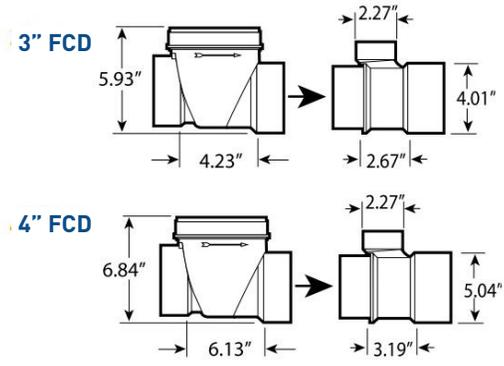
Notes: ACCESSIBLE FLOW CONTROL DEVICE (FCD) IS SUPPLIED FOR INSTALLATION UPSTREAM OF THE GREASE INTERCEPTOR (GI) - 3" or 4" INLET/OUTLET MODELS
