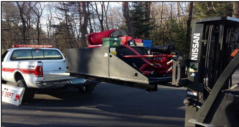
In early December, we took delivery of a new skid tank that slides into the back of a pickup truck to be used for fighting brush fires. The unit includes a 250 gallon water tank, a 200 gallon per minute water pump, and a 20 horsepower gasoline engine. This unit replaced one that was aging and unreliable. This skid tank is similar to other specialized fire equipment, we may not need it often, but when we need it there is nothing else
