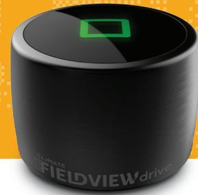
The FieldView™ Drive is an in-cab hardware device that plugs into your equipment's CAN diagnostic port, capturing both machine and field data. It connects your equipment to your iPad® via Bluetooth®, monitoring and displaying data as you pass through your fields.
