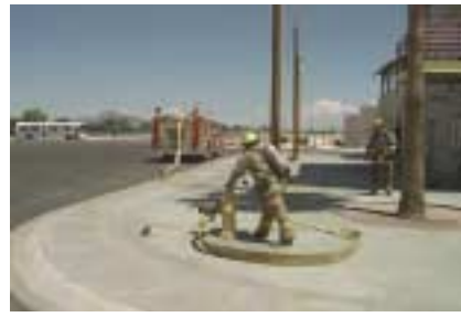
(Fig. 2.16b) The same pumper completing the straight lay towards the fire scene, and a firefighter preparing to operate the hydrant after the hose is safely laid out.
