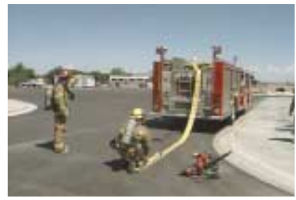
(Fig. 2.16c) Pumper performing a reverse hose lay from a fire scene (to feed the monitor nozzle shown) towards a hydrant.
