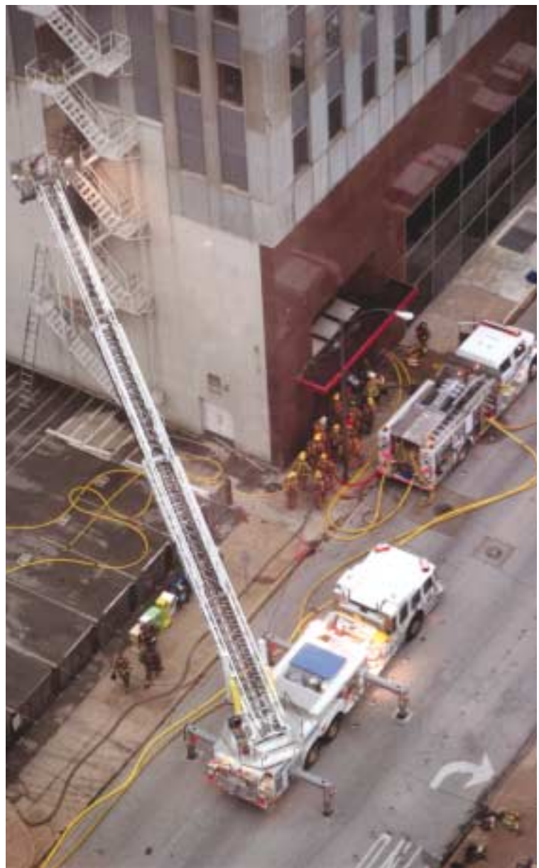
(Fig. 1.2) A view from above of both a pumper (top) and an aerial apparatus (bottom), in this case a platform type of aerial.
