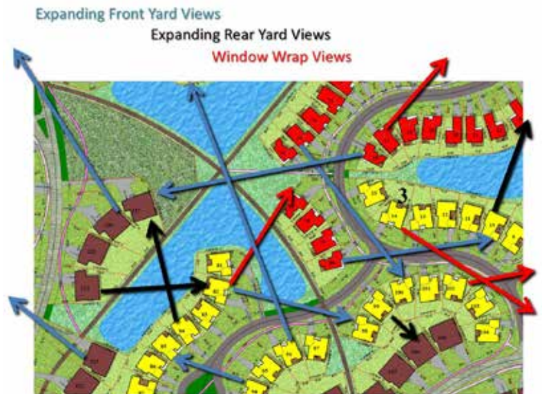
Figure 6: Angle relationships between homes of a curved design increase the length of views from within the homes.
