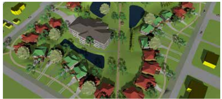
Figure 1: A redevelopment study using coving. Note how the homes undulate in and out forcing non-rectangular lots
