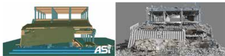
INACHUS collapse simulation software model (left) and scan of collapsed structure.
