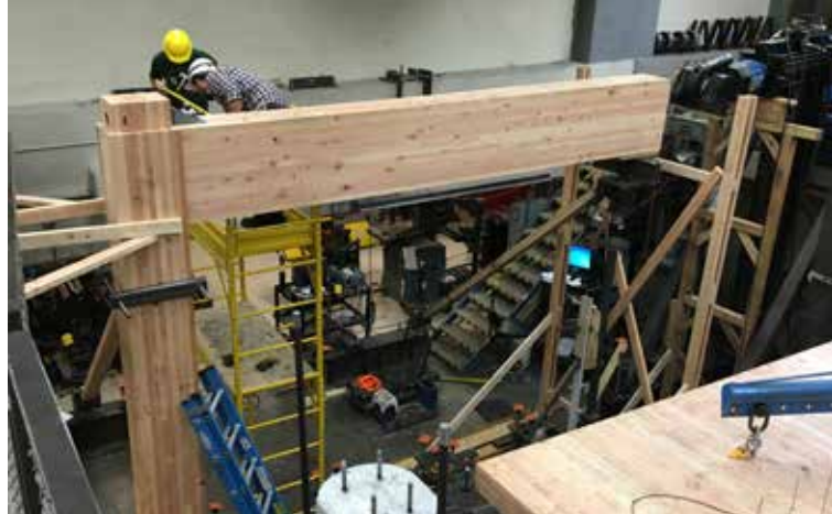
Mass timber beam-to-column seismic testing at Portland State University. Photo: courtesy of KPFF Consulting Engineers
