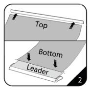
2. Attach Velcro strips to the top and bottom of the back of banner.
