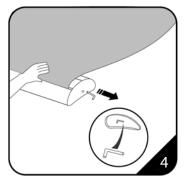
4.Peel off the cover, remove the screw underneath the chrome end of the base and detach. Then, with the graphic held firmly, carefully pull out the retaining pin, then put it into the cover.
