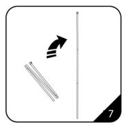
7. Unfold the pole and slip the pieces together to assemble it to a rigid pole (the hooked end corresponds to the top and the round end belongs to the bottom base).
