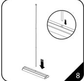
The bottom of the assembled pole slides into the round socket in the centre of the base unit.
