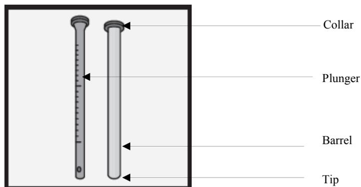
1. Push the plunger all of the way into the barrel.
