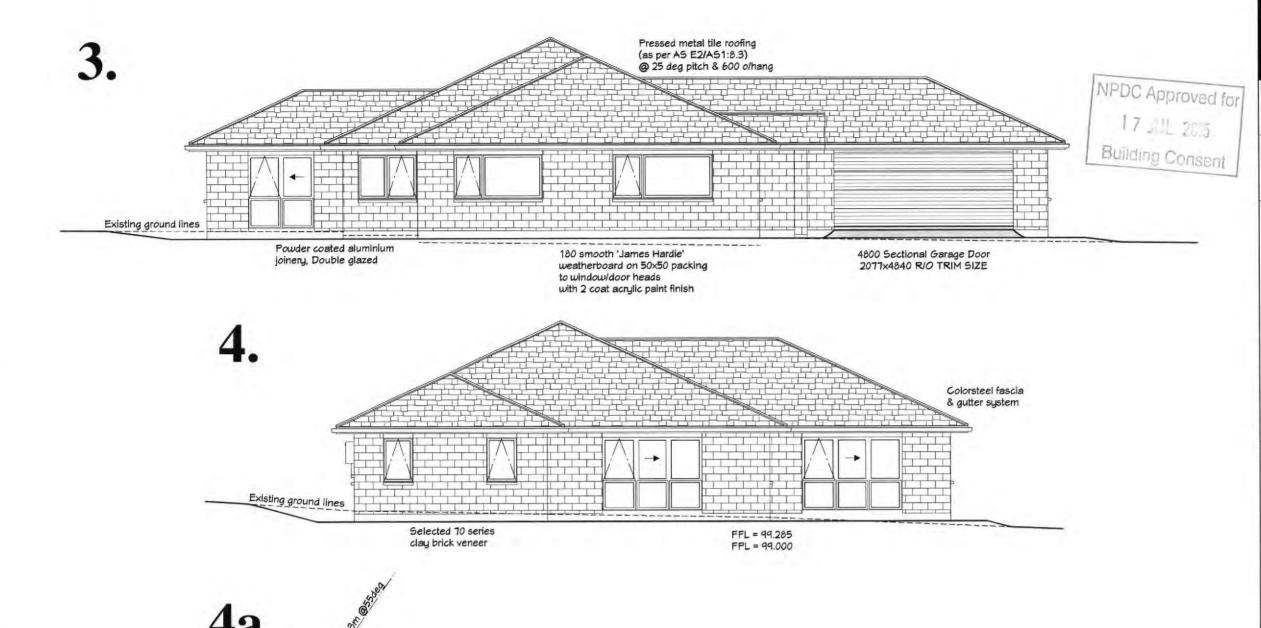
Refer to site plan for elevation reference
