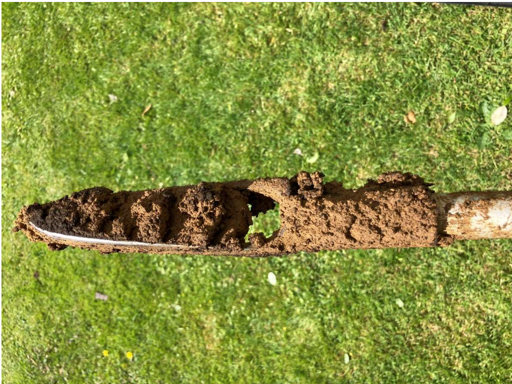
PHOTO 8: Moisture increase in silty Taranaki ash.
