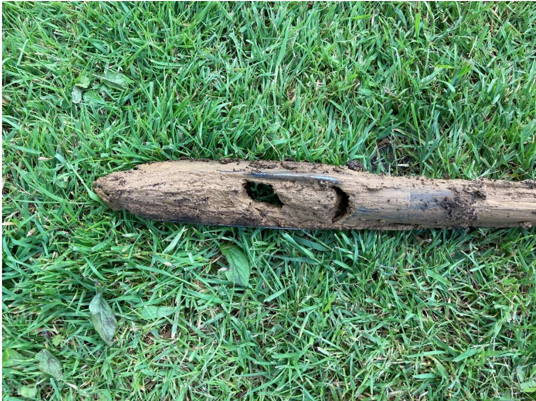
PHOTO 9: Light grey brown silty ash at 2.7 metres depth.
