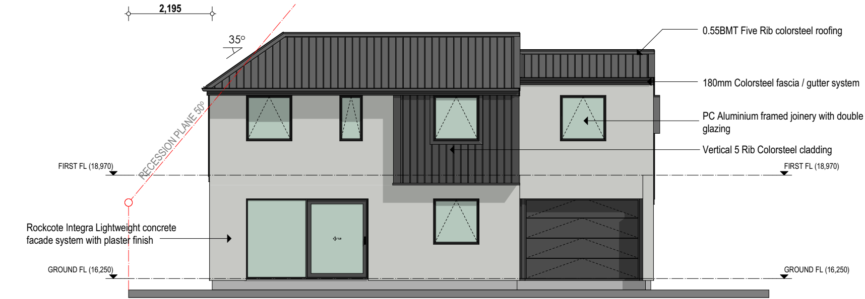
2 North West Elevation
