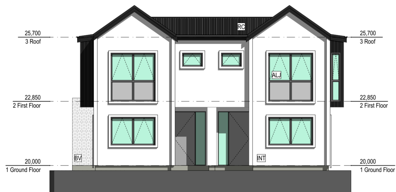
3 UNITS 1 AND 2 SOUTH ELEVATION 1:100
