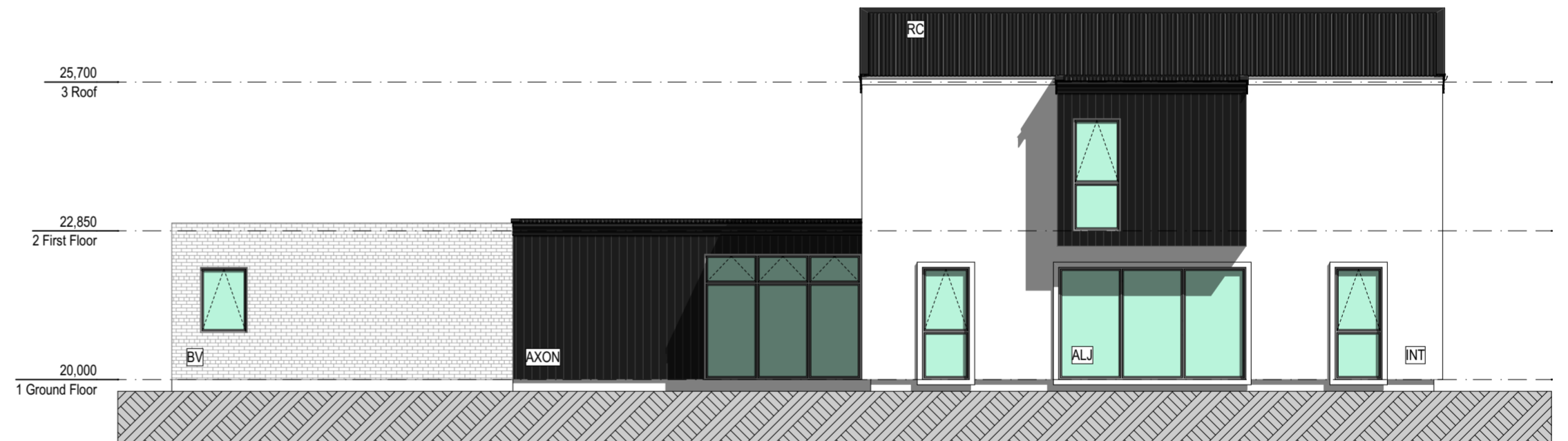
4 UNITS 11 AND 12 WEST ELEVATION 1:100
