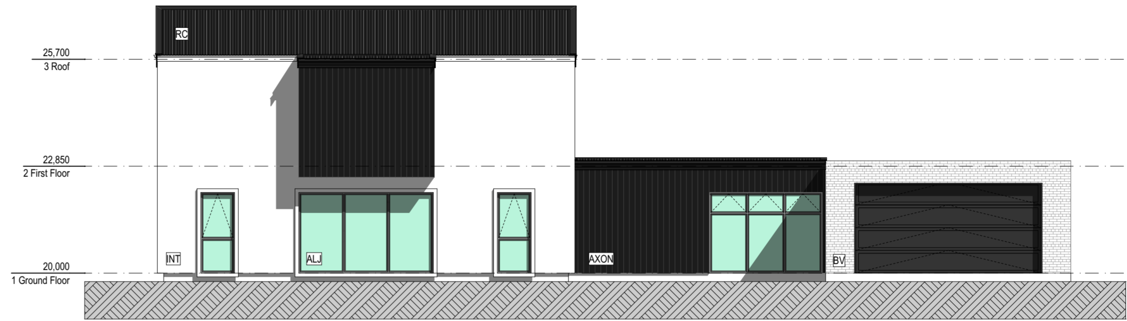
3 UNITS 11 AND 12 EAST ELEVATION 1:100
