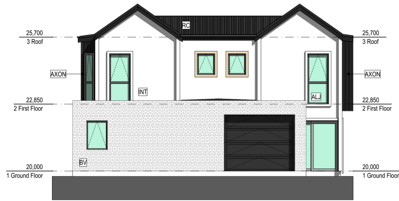
1 UNITS 11 AND 12 NORTH ELEVATION 1:100
