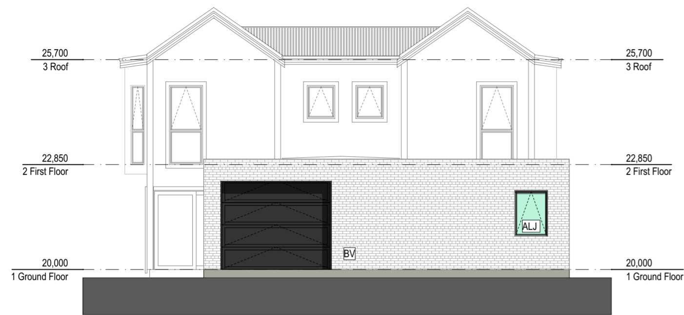
1 UNITS 1 AND 2 NORTH ELEVATION 1:100
