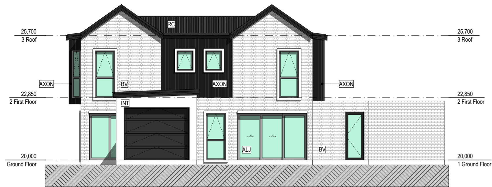
1 UNITS 5 AND 6 NORTH ELEVATION 1:100
