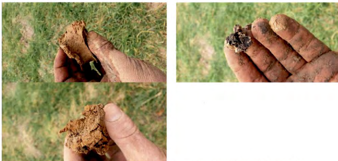
Figure 4: Typical soil samples from boreholes (note discolouration from the typical Taranaki Ash)
