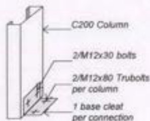
BASE CLEAT SINGLE COLUMN (Detail 07)
