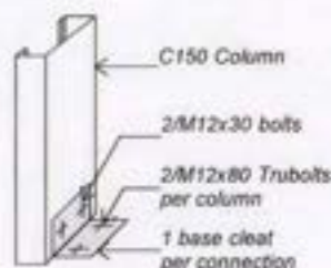
BASE CLEAT SINGLE COLUMN (Detail 07)
