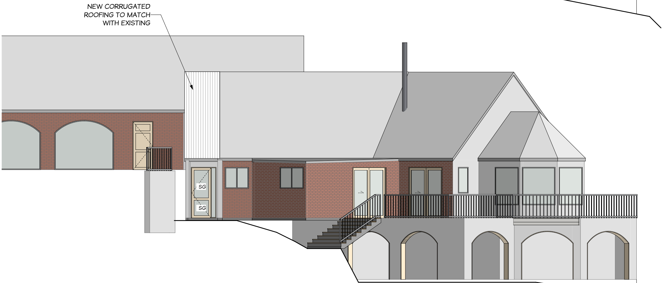
ALTERED PART NORTH WEST ELEVATION 1:100
