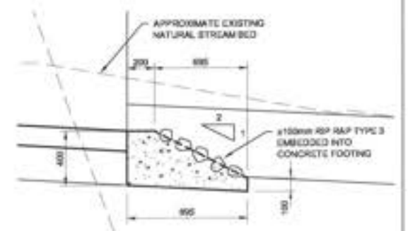
CONCRETE FOOTING DETAIL 1 SCALE: 1:20[A1] 1:40[A3]
