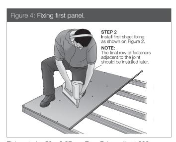
Fixings to be 50 x 2.87mm RounDrive nails at 200mm maximum centres
