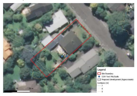
Figure 3: Site testing locations relative to approximate build location.
