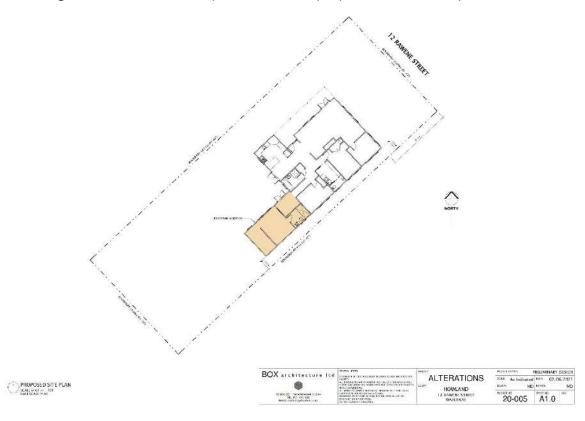
Figure 1: Development plan as supplied by Box Architecture Ltd (Sheet A1.0) showing the rear extension with master bedroom and ensuite.
