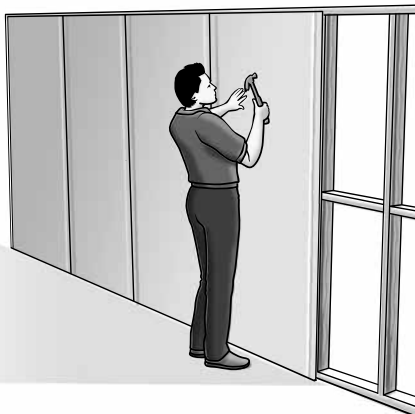
Figure 4: Fixing remaining sheets
