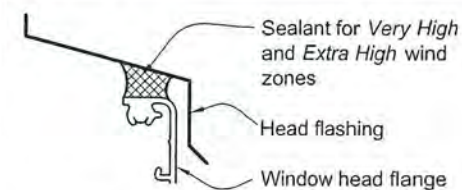
(c) METAL HEAD FLASHING SEALANT FOR VERY HIGH AND EXTRA HIGH WIND ZONES
