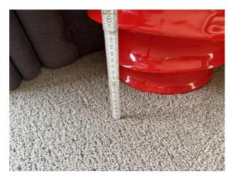
Photo 21 Reading is 105mm, making it 10mm lower than the datum level, this is within reasonable tolerance.
