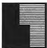
PURLIN LAYOUT (MAX 1200 crs.)
