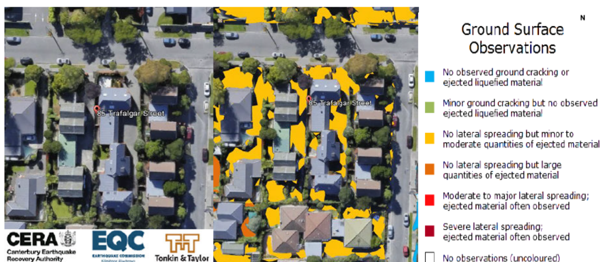
Photo 3. EQC liquefaction and lateral spreading observations obtained from Canterbury Geotechnical Database show “No observations (uncoloured)” following the September 2010 and “No lateral spreading but minor to moderate quantities of ejected material” following the February 2011 earthquake events.
