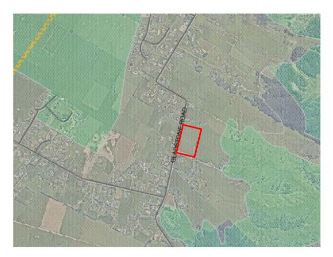
Above is an excerpt from the HDC liquefaction risk hazard mapping showing where the Q2a alluvial deposits between Tararua Road and Queen Street are identified as liquefaction risk unlikely and the location of the Poulton property immediately to the East. Below is the site specific Geology for 167 Gladstone Road as mapped by GNS NZ: data.gns.cri.nz/geology & 1:250,000 Geological Map 10, Wellington.
