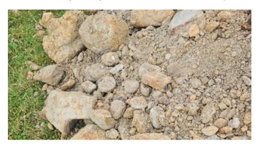
Table 2: Test Pit 2 & Scala I, Lot 1, 169 Gladstone Road. Soil classification as per the Field Description of Soil & Rock – NZ Geotechnical Society Inc, Dec 2005
