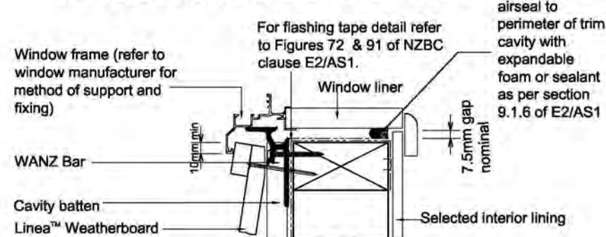
WINDOW SILL DETAIL Scale 1:5
