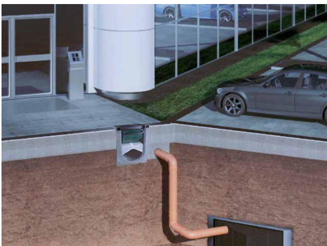
Figure 3. Groundwater infiltration using a FlowGuard to treat stormwater runoff
