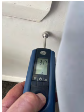
There were two elevated wet moisture readings in the bathroom noted which could be from condensation buildup in the corners of the timber window reveals and sill. This should be further investigated to determine the cause and make good.
