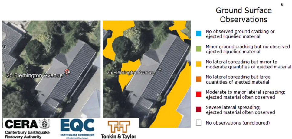
Photo 3. EQC liquefaction and lateral spreading observations show “no observations (uncoloured)” following the September 2010 earthquake event and show “no lateral spreading but minor to moderate quantities of ejected material” following the February 2011 earthquake event. Site specific bearing verification investigation was undertaken as part of this assessment.
