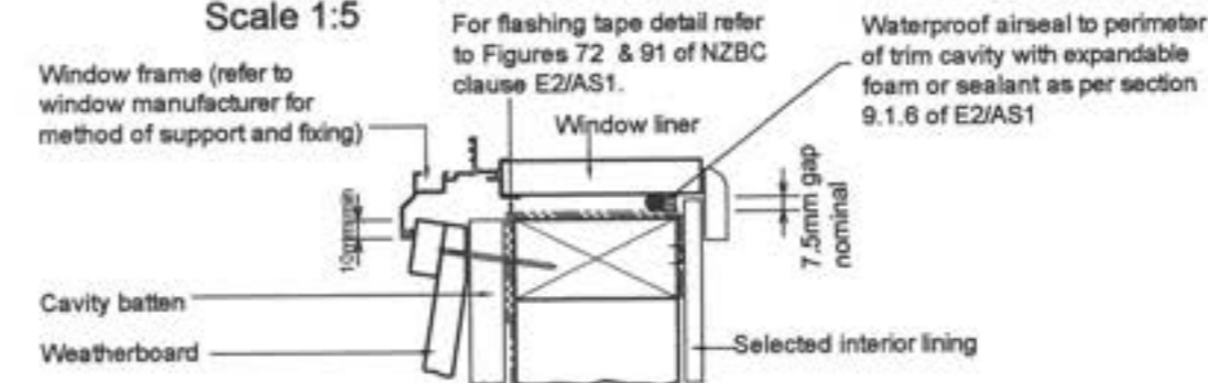
WINDOW SILL DETAIL Scale 1:5
