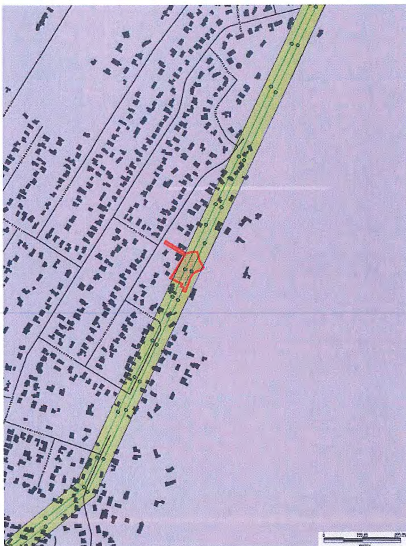
Figure 8: GIS image showing A & B transmission lines and dwellings (shaded 'blocks'). The shaded corridor represents the 20m 'proximity zone' established by the District Plan – measuring 20m from the centre line of each transmission line (i.e. not each conductor but from the centre of the A & B lines as a whole). For simplicity's sake, the centre point for the A & B lines has been measured from the poles as these are typically situated in the centre of each line.
