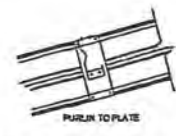
TYPICAL PURLIN TO RAFTER DETAILS
